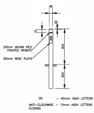
**DETAIL 3- VALVE INDICATOR POST DETAIL**
