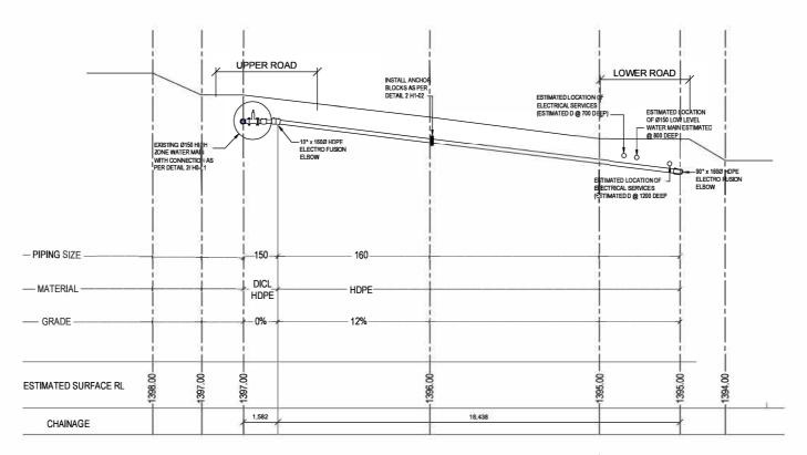
DETAIL 1- SECTION A-A (STEEP WATER MAIN SECTION)
